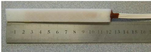
**Figure C.2. Embedded strain gauge for monitoring shrinkage deformation**
