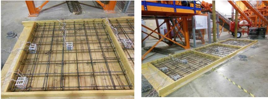
**Figure C.1. Slab section used for shrinkage deformation evaluation**
