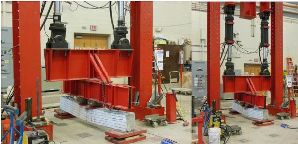
**Figure C.18. Beam flexural test setup**
