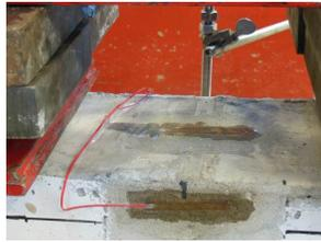
**Figure C.20. Installation of LVDT (left) and strain gauges on surface of concrete beam (right)**
