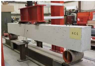
**Figure C.28. Photograph of beam shear test setup**
