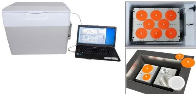
Figure A.12. Isothermal calorimetry used for hydration kinetics of mortar
