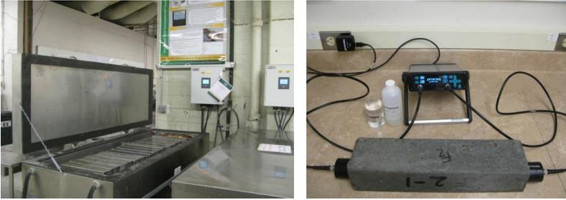
**Figure A.19. Freeze-thaw chamber (left) and ultrasonic velocity instrument (right)**
