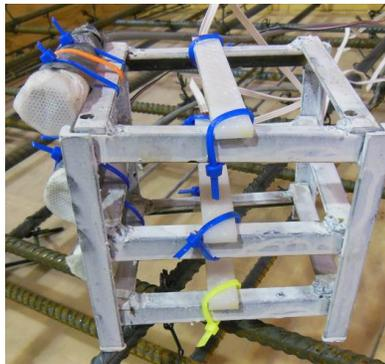
**(a) Layout A: 3 embedded strain gauges in longitudinal direction, 3 thermocouples and 3 relative humidity sensors**
