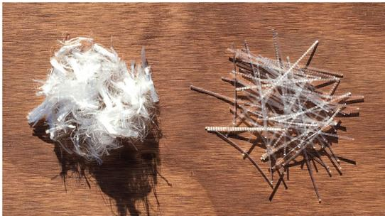
**Figure A.8. Micro (l) and macro (r) synthetic fibers**
