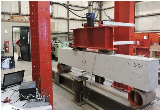
**Figure C.32. Photograph of beam splice test setup**
