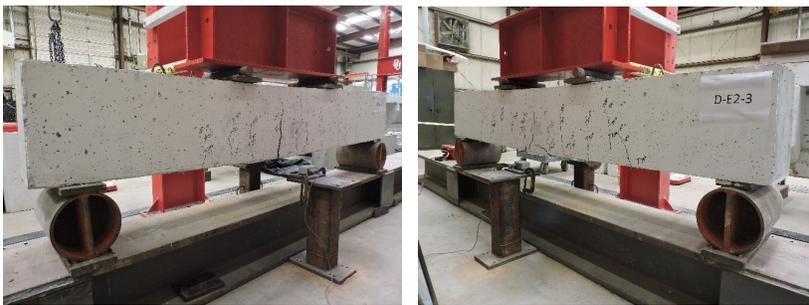
**Figure C.34. Typical beam splice test specimen failures**
