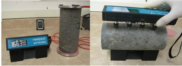
**Figure 2.3. Bulk electrical conductivity (left) and surface resistivity (right)**
