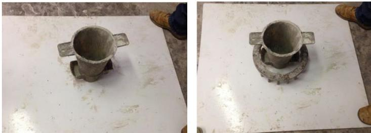
**(a) Slump flow test**
