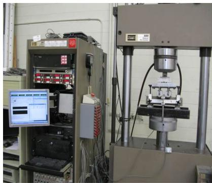
**Figure A.17. Test setup for flexural toughness measurement of FRC beams**
