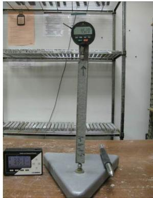
**Figure A.16. Drying shrinkage measurement of mortar**
