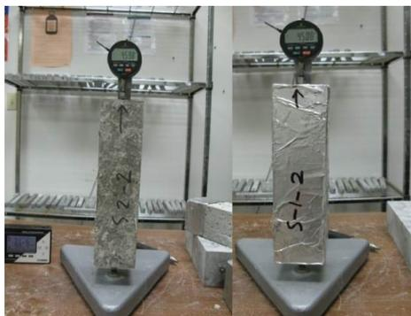
**Figure A.21. Shrinkage measurement of unsealed (left) and sealed specimens (right)**
