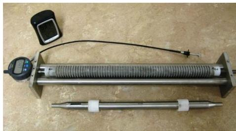
**Figure A.14. Autogenous shrinkage measurement device**
