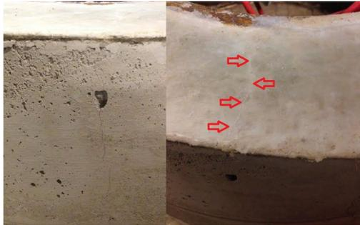
Figure B.6. Visible crack in PPE 0.00 mixture ring 2 from the side and above
