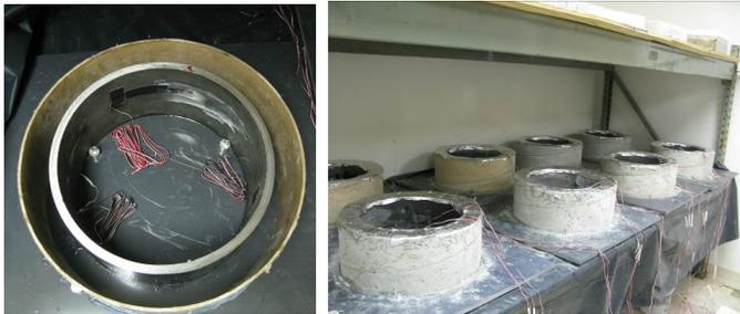
**Figure A.22. Restrained shrinkage ring test setup**
