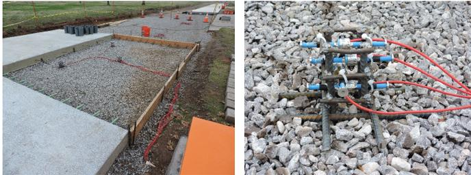
**Figure C.14. Vibrating wire strain gauge overall layout and close-up of tree No. 1**
