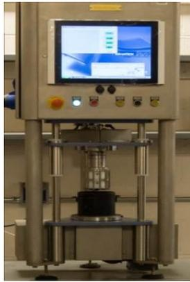
**Figure A.13. Coaxial cylinders rheometer used to determine rheological properties of mortar**
