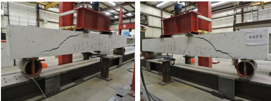
**Figure 4.2. Typical beam shear test specimen failures**
