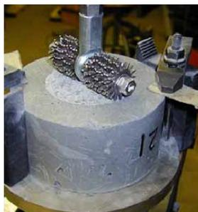
**Figure A.18. Abrasion resistance test setup**
